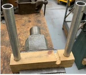
The fixture consists of two 6-inch lengths of electrical conduit and a block of wood. I drilled two  $\frac{3}{4}$ -inch holes halfway into the block to hold the conduit. They are a snug fit but do wobble. I also drilled a  $\frac{1}{2}$ -inch hole on the flank and then sawed from the top to create a channel.
