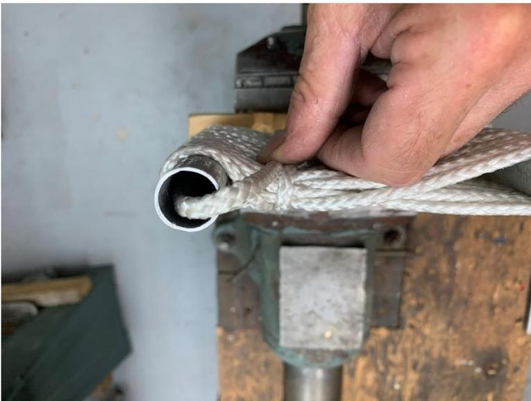
While holding the line with my thumb, I feed the end down the post.
