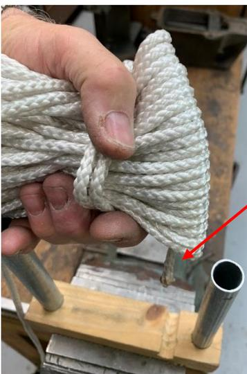
As I lift the bundle off of the posts, the end of the line can be seen extending out the bottom.
