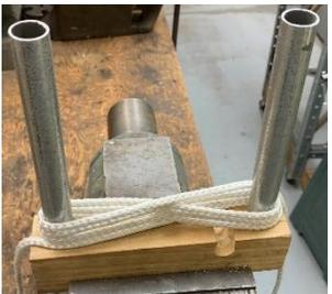
I loosely form my figure 8s. Even then, there will be enough force on the posts to cause them to tilt in a little. This is a feature and not a bug. This will make it easier to lift the bundle off of the posts.
