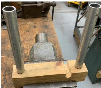
My solution is to make a fixture to provide the extra hands. This is a proof-of-concept, so it is not pretty. Yet it does work well. The final iteration will not need to be mounted in a bench vise.
