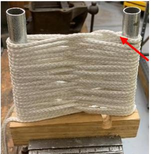
I'm done coiling the line. Note that the end of the line runs around the right post and then over the backside of the bundle.
