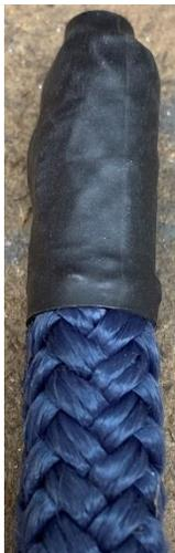
I slid on a length of heat shrink and applied my heat gun. It solidly compressed the end of the line plus locked in at the transition to soft line. There are no burn marks visible.
