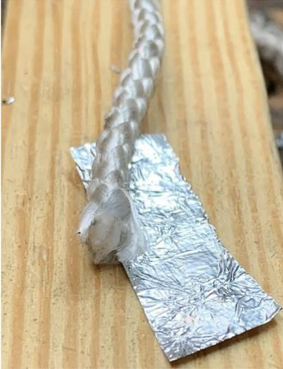
I start with a piece of aluminum foil. The width is about three times the diameter of the line. The length should be enough to wrap around the line a few times.
