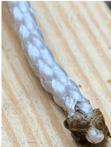
A common remedy to the little cloud is to roast the end over a flame. This melts the plastic and forms little blobs. The line is sealed, but you may have some sharp ends to contend with. They can hang up on the line while tying knots.
