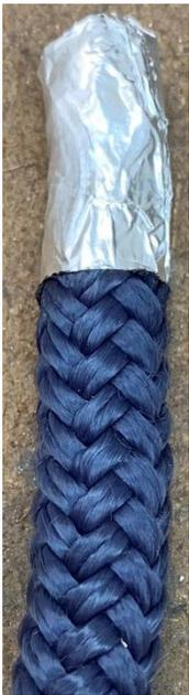
I have a piece of 1/2-inch line. After wrapping it in foil, I heated the end with my butane torch being careful not to burn the exposed line.
