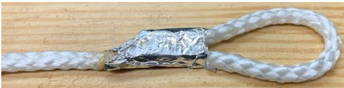
Much to my surprise, the joint felt solid. I pulled “hard” on the loop, and it held. When I pulled harder, it did break. Reflowed plastic is not that strong.
