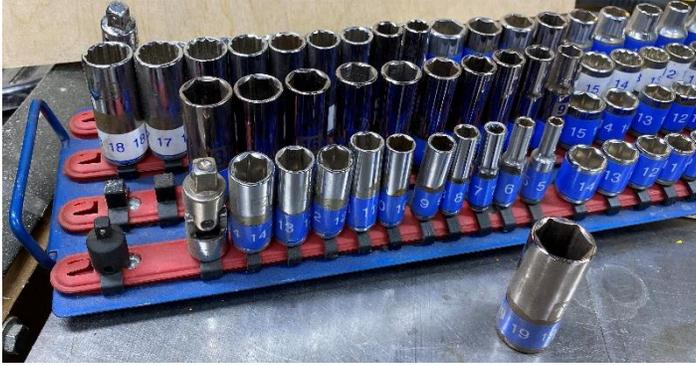
For the way I work, I like taking an entire set of a tool type to the work. I hang the socket board on the outside of my toolbox to increase direct access and to conserve space in the drawers. On the board, there are separate socket rows for 1/4", 3/8", and 1/2" drive. The large labels on each socket are MUCH easier to
