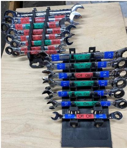
For ratchet wrenches, I wanted a clearer indication of the direction for tighten vs loosen. Hence the green "On" and red "Off" labels on opposite sides of the wrench. (*Editor's note: I appreciate having the color and text because I will forget the meanings of the colors.*)
