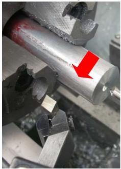
I turn metal on my lathe. The stock spins counterclockwise as viewed from the tailstock. When I want to cut starting from the right and moving left, I use a left hand cutter as shown here.
