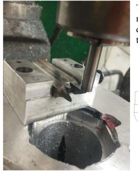
This article presents both the hardware and G-code needed to machine this part. It is 0.250 inch in diameter and 0.293 inches long. I'll need 102 of them before I am done.
