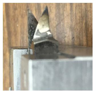
In this side view of the cutter block, you can see a left hand cutter in the background and a right hand cutter in the foreground. The left hand cutter forms the hemisphere and the right hand cutter does the reduced diameter section and parts off.
