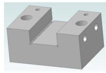
It is secured to the hex fixture using two SHCS <sup>1</sup>/<sub>4</sub> -20 and two dowel pins. The pins provide accurate position relative to the base
