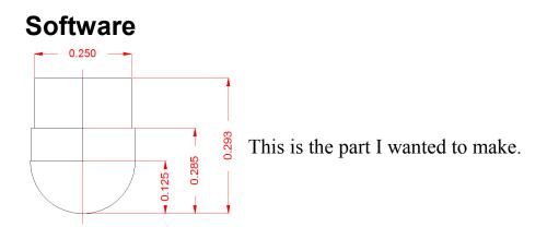
From a software standpoint, I am making this. That red vertical line is my COR which is aligned with the Z axis. I am sighting along the X axis in a negative direction so see the Y axis pointing to the right. It is pointing towards the column of the mill.
