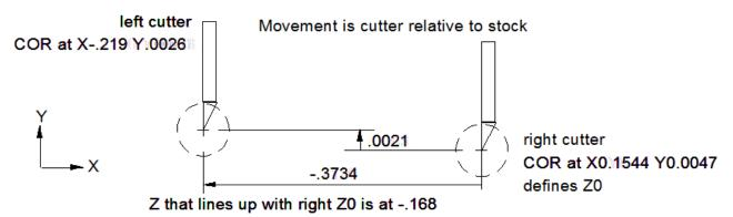
Calibration was time consuming but is only needed after disturbing the cutters in the cutter block.
