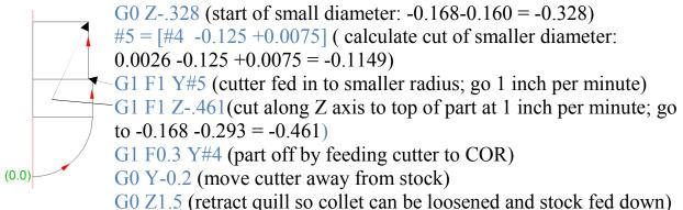
G0 X#1Y#2 (move back to first cutter so COR is centered at point of right cutter) M30 (end of program; rewind to start)
