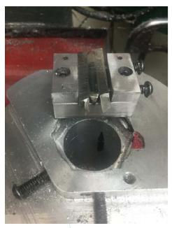
I used a 1" x  $1\frac{1}{2}$ " X 2.1" block of 6061 aluminum to make my cutter block. More on how I machined it later.
