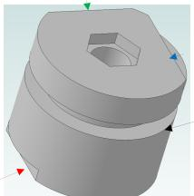
The hex fixture has three flats machined into it used for reference. In its base is a flat (red arrow) that is set parallel to the Y axis as part of its installation.
