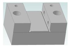
Then I CNC cut the recess that would take 3 cutter blanks. The recess is 0.8 inches wide and 3/8 inches deep. A light cut was made across the front face of the block to define my front reference surface. This face is aligned with my X axis and will be used during set up of the cutters. After removing the block, the inside corners of the recess were relieved with
