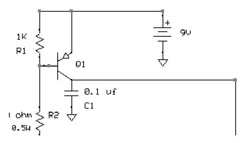
This function is performed by having the test current pass through R2. This causes Q1 to be driven deep into saturation. Q1's collector is then pulled up to near 9V which feeds the quad op amp.
