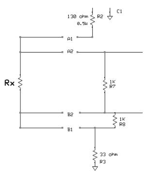
The test current passing through R2 feeds into the unknown resistance,  $R_x$  via probe A1. The current then flows out of  $R_x$  via probe B1, into R3, and returns to ground.
