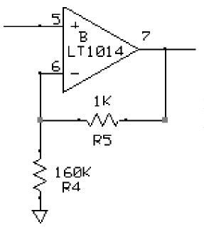
Next look at op amp B in the ideal case. The voltage on pin 5 essentially equals the voltage on pin 6.
