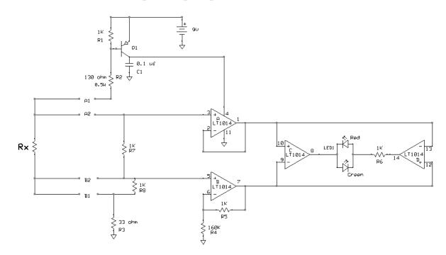
First consider op amp A in the ideal case. This op amp is configured for unity gain. The output voltage equals about  $10^5$  times the input voltage. This means that the input voltage is  $10^{-5}$  times the output voltage. So for any output voltage, the input is extremely tiny. We can therefore say that V<sub>3</sub> approximately equals V<sub>2</sub>. But pin 2 is tied to pin 1 so the output voltage essentially equals the input.
