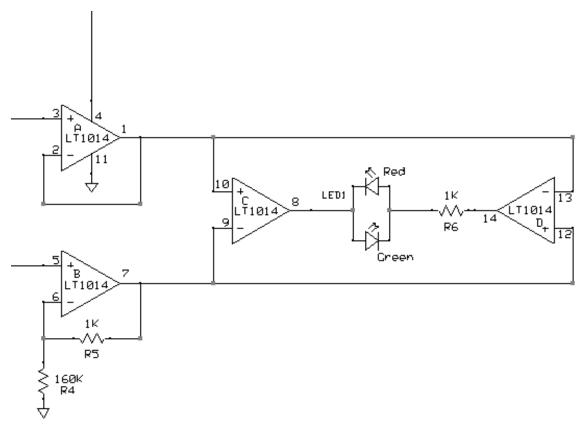
When  $R_x$  is above the threshold, the voltage on pin 1 is greater than the voltage on pin 7. This causes op amp C to drive pin 8 to near 8V while causing op amp D to drive pin 14 to near 0 volts. Current then flows from pin 8 to pin 14 causing the green LED to light.
