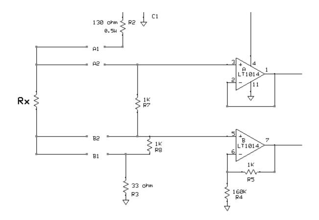
Op amps A and B measure the voltage across  $R_x$ . When  $R_x$  equals the threshold, the voltage at pin 1 equals the voltage at pin 7. Below this threshold, the touchdown LED is red. Above this threshold it is green.
