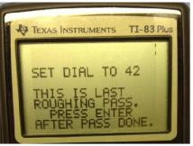
The program then says to turn the dial to 42 in preparation for the second roughing pass. This will ideally reduce the diameter from 1.4" to 1.3". If we took another roughing pass, our diameter would ideally be 1.2" and that is too small. So the program tells us that this is our last roughing pass<sup>3</sup>. When done with this roughing pass, I press ENTER.
