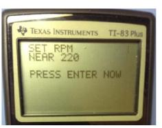
The program takes the average of the goal diameter and current diameter plus the specified SFM to calculate the RPM.
