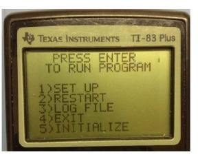
When the program starts up, it offers the user the options of running, changing the set up parameters, viewing the log file of the previous session, exiting, or doing a one-time initialization. I have previously used SET UP to tell the program that my roughing depth of cut (DOC) is 50 and I want to make 1 outside diameter (OD) finish pass. It was also told that my in-feed dial has a maximum value of 100. My Surface Feet per Minute (SFM) was set to 80 for steel and 100 for aluminum.
