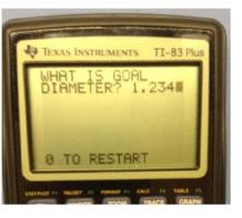
The user is then asked for the goal diameter. They can back space or move to any digit to correct the entry. When done the user presses ENTER. I have entered "1.234".
