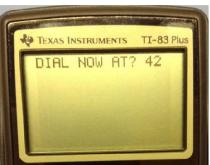
The user moves the cutter until it contacts the workpiece. The program asks the position of the dial.
