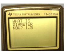
The user is next asked for the current diameter. I have said "1.5". The program now has enough information to know if this is an OD or inside diameter (ID) being turned plus how many roughing passes to make before measuring for the finish pass. Given a starting diameter of 1.5" and a goal of 1.234", I have to reduce the diameter by .266 so must feed the cutter in by .133 because my lathe is set up so dial movement is related to radius and not diameter.
