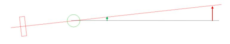
Say I had to zero my instrument at some distance from the pivot point and then move to the end of the leadscrew for my second reading. Rotating the leadscrew until I again see zero isn't going to work. This is because my zero point is not at my pivot.
