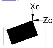
The challenge is to locate the corner of a tilted block in a mill vise without a special tool.
