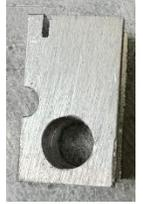
I did have one minor annoyance. The hot rolled steel was not squared up on the edges. I used my disk sander to cut a flat area for the plate, but this put the plate about 0.075 inches above the vise ways. I had to add a shim it to bring the plate's face level with the ways.
