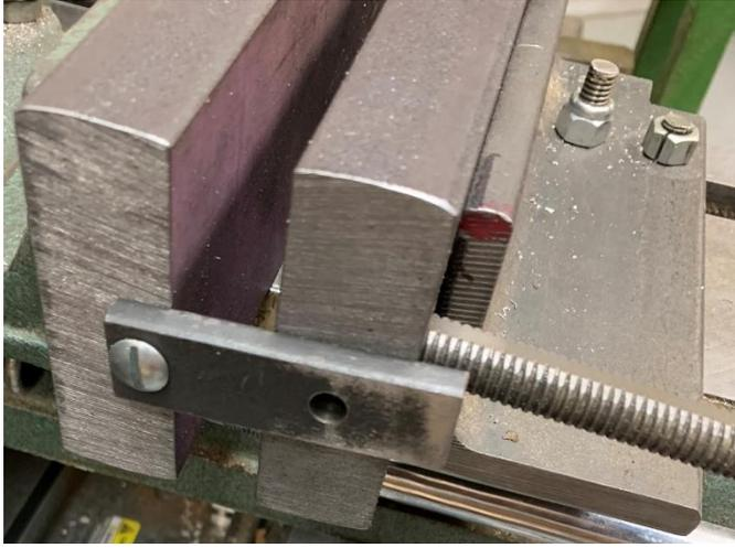
After sleeping on this idea overnight, I decided I wanted a better way to align the movable jaw to the fixed jaw. I bolted a bar to the end of the fixed jaw. I used a Belleville washer so I can swing the bar up as needed.
