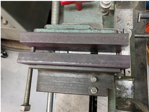
There are times when I need to saw a small bit of metal in my bandsaw, and the jaws do not extend close enough to the blade.
