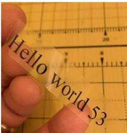
The procedure transfers images printed by a laser printer onto packing tape. If you have a color laser printer, so much the better. The key think to understand is that the toner is applied to plain paper in the printer. The process transfers that toner to the tape.
