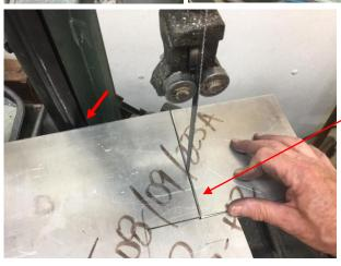
As with all machines, there are limitations. In this case, my plate has hit the support arm of the saw before the cut is done (red arrow).
