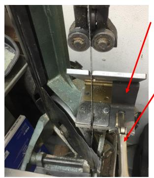
The trick is to pivot the table up 45°. Note the piece of scrap angle under the table on the right side clamped in place with a Vise-Grip.
