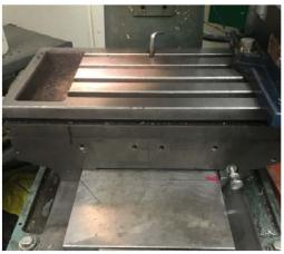
By drilling one hole, I am able to access the Y take up nut without disturbing the X axis. This hole enables me to feed an allen wrench through the table and into the top of the Y axis take up nut's Socket Head Cap Screw.
