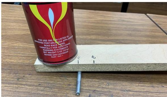
First, I put the full canister over the disk with the rod under the board. I rolled the board back and forth until it balanced. I then put a line on the board labeled with “F.”
