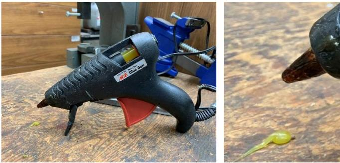
I have used a hot glue gun for decades. I prop it up on its stand and glue drips out while it waits to be used. No surprise there – gravity acts on the molten glue in the nozzle and it drips out.
