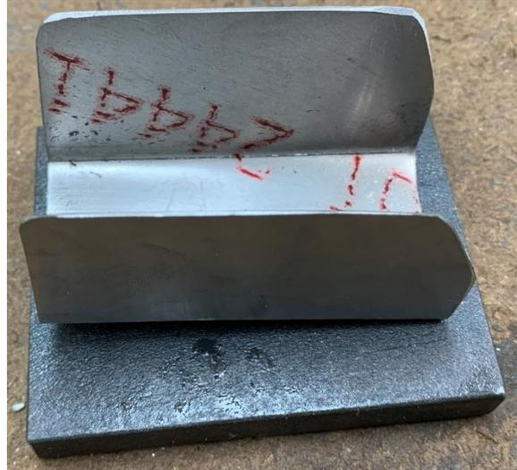
I bent up some tempered aluminum sheet stock and bolted it to a scrap of hot rolled steel. It was secured at one end with a 6-32 into a tapped hole. The other end has a longer 6-32 with a spacer to provide a slight angle. It too screwed into a tapped hole.
