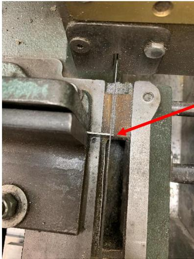
My 4 by 6 Horizontal/Vertical bandsaw is great for holding and cutting large stock. But when faced with cutting tiny bits of material, it needs some help. Those big jaws do not extend out to the blade so this thin stock tends to vibrate and bend due to the cutting force.
