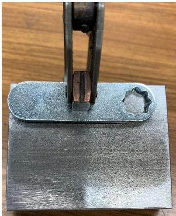
The front jaw is a block of metal the same length as the angle and 2 inches wide. It is  $\frac{1}{2}$  inch thick.
