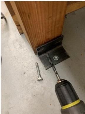
With the workbench back in the desired position and the bracket secured to the floor, I used the drill that matches the body of the screw. Remember that I last used this drill to open out the two adjacent holes.
