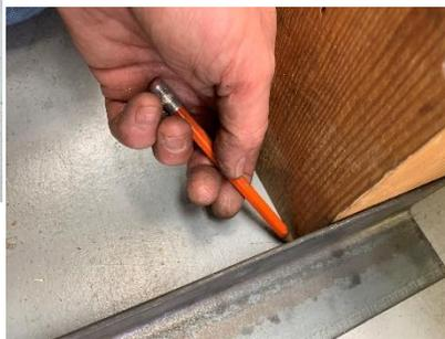
I started by slapping some angle stock against the first leg of the bench. I don't care about its cut length, just want it to match the leg. So a quick mark with a pencil is precision enough.
