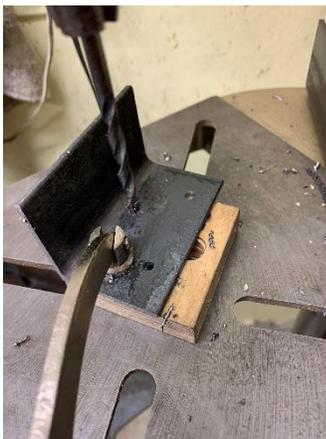
I located the second hole by eye. It should be "pleasingly close" but, again, the exact position is not important. Ultimately, this hole will also pass a lag screw.
