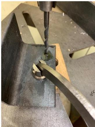
Moving over to my drill press, I drilled my first hole with a 3/16 bit. Eventually, this hole will pass one of two lag screws. The location of the hole looks about right but I couldn't tell you its exact position.
