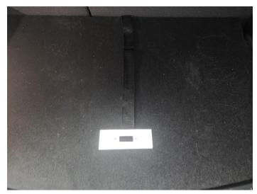
Folding the strap into a loop, I fed it through the slot in the plate and around the bar. Then I loosely secured the bar with flat head screws plus washers between the bar and the plate.
