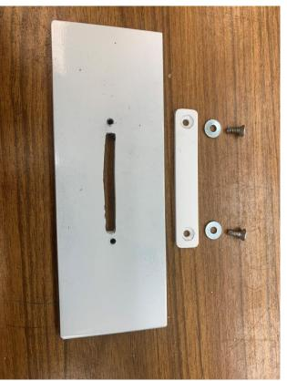
I fabricated a plate from 3/16-inch thick aluminum.
