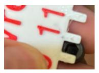
To use the gage, I place the gap over the hex hole and then read off the number of 64ths. In this example, I need a  $\frac{10}{64}$  inch =  $\frac{5}{32}$  inch hex wrench.
