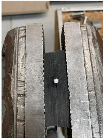
While steel vise jaws grip the sides of a piece of stock, rubber jaws wrap around it. This added support permits the user to apply force parallel to the vise jaws and not just perpendicular to it. There is also little chance of marring the stock.
