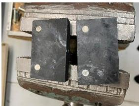
Each slab of rubber has two 1/4 inch diameter holes drilled in them with an end mill. The holes are deep enough to accept 1/8<sup>th</sup> inch thick neodymium magnets. I put a dab of adhesive in each hole and pushed in the magnet.
