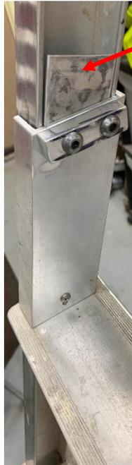
Then I raise up the top end until the lower tab drops into the space next to the lower step (blue arrow).
