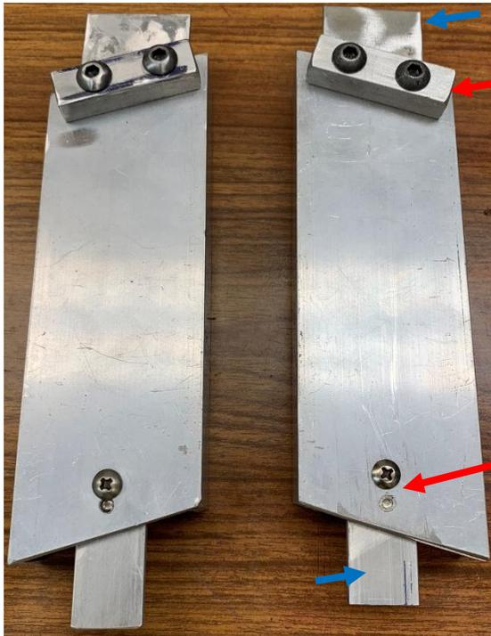
The left and right vertical supports rest on the lower step. The half-step rests on these chocks that are secured with 1/4-20 bolts. The tabs (blue arrows) at the top and bottom lock these verticals to the flanks of the ladder.
