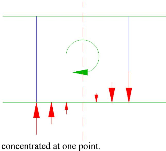
Consider our plate with a rotational force again in the center. This time the plate is sandwiched between the two walls, shown as green horizontal lines.
