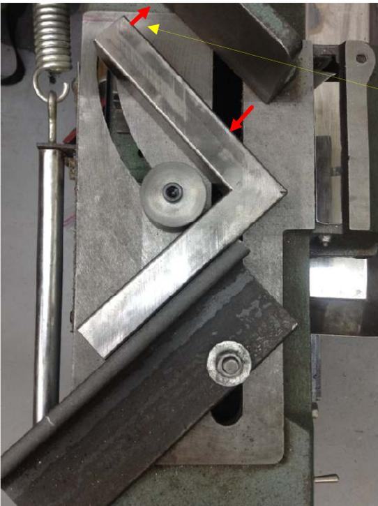
The end of the fixture will move towards the fixed jaw while closer to the 90° corner, the fixture moves away. This does not produce a usable clamping force.
