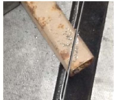
With insufficient offset of the pivot and movable jaw bolt, the workpiece did shift.
