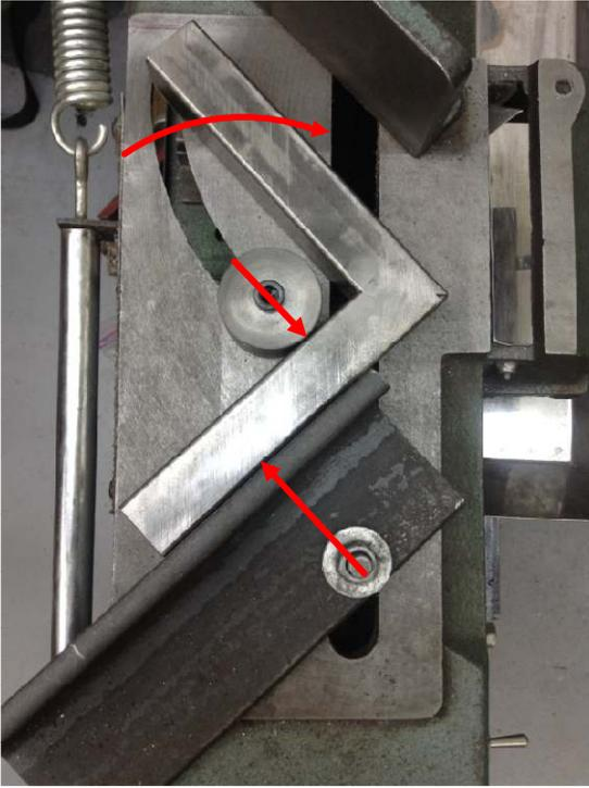
Looking at both vectors at the same time, we see that they do not line up. This causes the fixture to rotate clockwise as the movable jaw is tightened.
