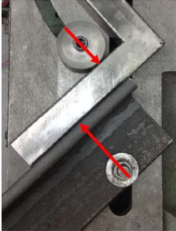
Remember that misalignment of force vectors? The larger this misalignment, the larger the twisting force. This actually helps us. If the vectors lined up, there is no tendency to rotate and no clamping force would exist between the fixture, workpiece, and fixed jaw.
