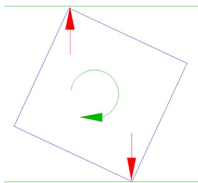
This might be clearer if you consider a square plate. Flanking the plate are two fixed walls shown as green lines. As I rotate the plate, the corners will move until they hit the walls. At this point, all of the turning force is
