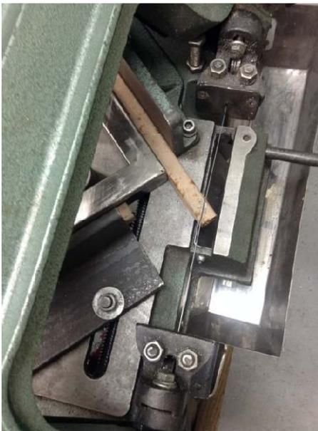
One solution is to build an attachment that permits both + and - 45° cuts with no change in saw set up or flipping of the workpiece. The picture on the left shows a -45° cut while the facing picture is +45°.
