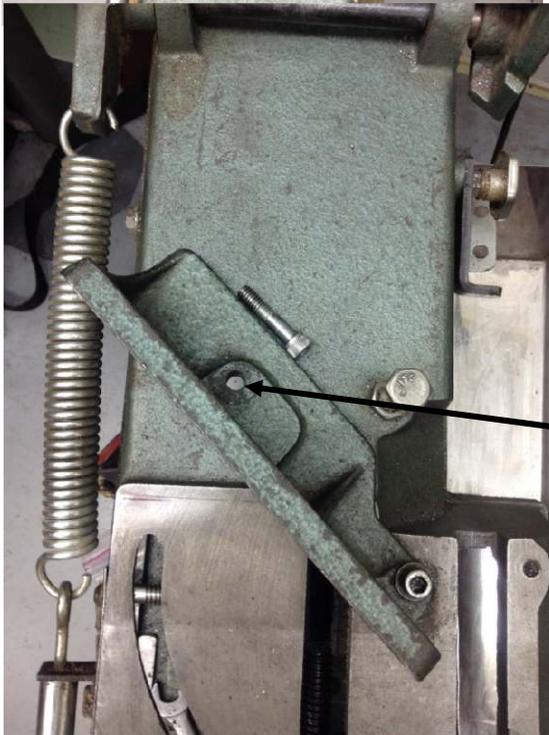
In preparation for installing the attachment, the fixed jaw is swung to  $-45^\circ$ . This requires me to remove the bolt that moves in the curved slot plus the nut that engages this slot from the underside.
