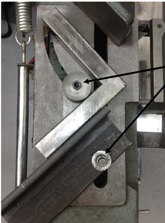
The nut is now under the base, the pivot is above it,
