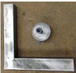
The attachment consists of two parts. One is a right angle fixture made of 16 gage 1" square tubing. The corner has been mitered, welded, and ground flat. The other part is a 1 ¼" diameter cylinder drilled to accept the hold down bolt.
