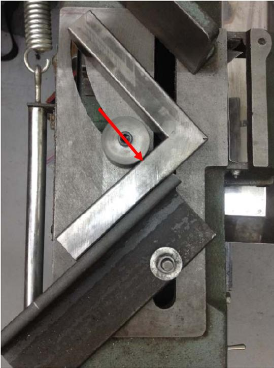
The first thing to understand is that when the cylinder presses on the fixture, the force will always be perpendicular to the surface of the bar and passing through the center. By using a cylinder, I get a smooth transition of this force vector as the fixture moves.
