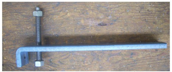
The mating piece fits over the movable jaw. The lower nut is Loctited<sup>©</sup> in place and acts as a thrust bearing. The upper nut is also glued in place and is my handle.
