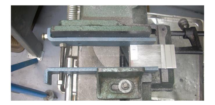
To use this attachment, back the threaded rod off until the block to be clamped is setting the distance between the extended jaws. Then turn the rod in until it matches this distance. Tighten the vise jaws and you are ready to cut.
