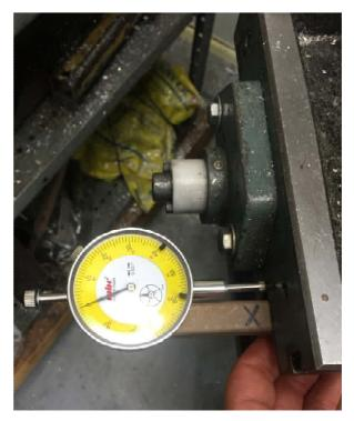
If/when I lose position, I just place my tool back into the ways and drive the table until the dial again reads 0.500. Then set the X DRO to -0.3836.
