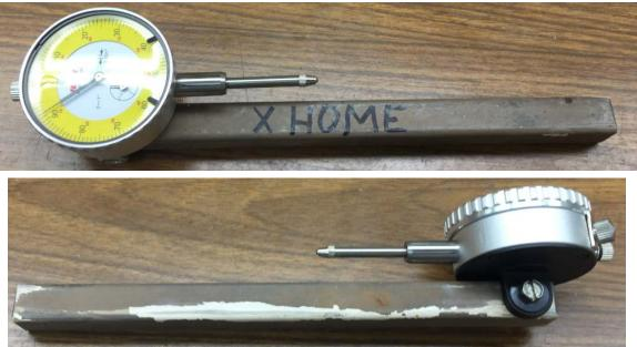
The ends of the tubing have been sawed square and sanded to a smooth finish. The rest of the tubing was lightly sanded to remove any burrs. The dial indicated is bolted to the tubing using a Belleville washer. This washer gives me enough pressure on the dial indicator lug to prevent unwanted movement yet still lets me make adjustments.
