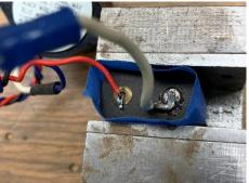
I built a mold out of 3M painter's tape and held it lightly in a small vise. I did bend the white wire so it exits out the top.
