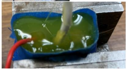
Working in layers, I fill up the mold. The trick is to not leave voids.
