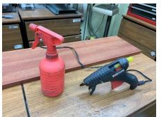
My hot glue guns is heating. I also have a fine water mist sprayer. It is handy if I need to speed up the cooling process.
