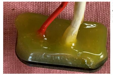
I then smoothed the edges with a *quick* burst from my heat gun. Too much heat and the hot glue will start to slump.
