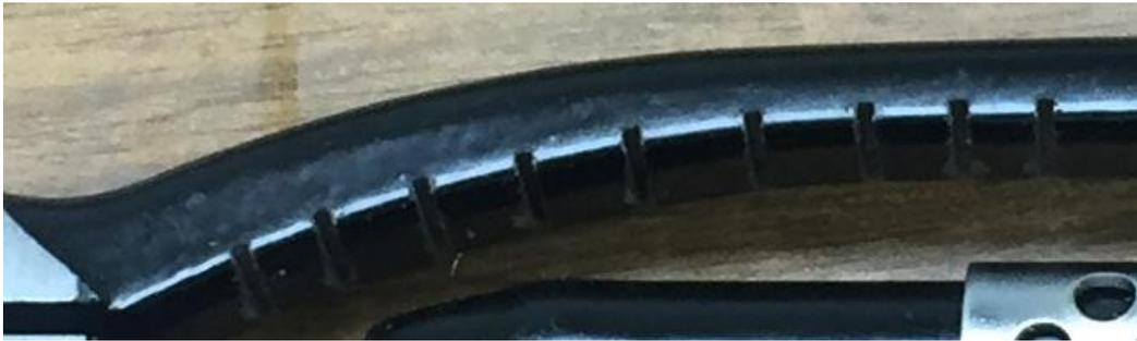
The cuts are about 1/16" deep every 3/16". The other handle is welded to the center rod so access was not possible.
