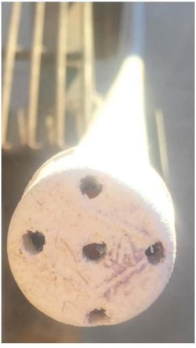
The other end of the pipe was terminated in a cap which had been previously drilled with an 1/8 inch drill.
