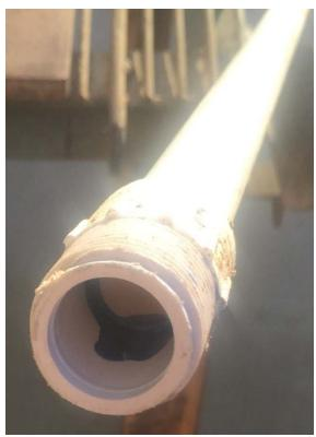
The hose coupler was cemented on one end of a 10 foot long piece of ½" Schedule 40 PVC pipe.
