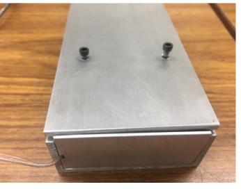
With the lid in place, I aligned the first screw with its hole in the circuit board. Then I started to turn the screw while pushing down. The nylon nut hung up on the top face of the circuit board so stopped turning. Then the screw fed in until it engaged the threaded hole in the bottom of the enclosure. When the head of the screw was snug on the top of the cover, I stopped turning. The second screw was fed in the same way.
