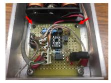
and also secure a circuit board that is inside. The red arrows point to the two anchor holes needing to be filled.
