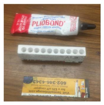
If you want to put a strip of flexible magnet on the bottom of a bar, you will need contact cement and a source of magnetic plastic. I have plenty of these magnets and never paid for any of them.
