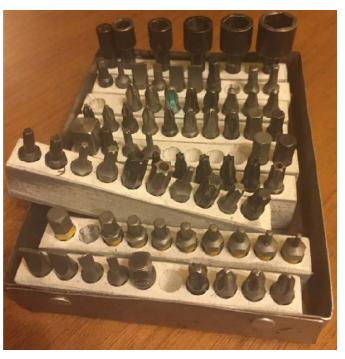
My solution was to make a set of ½" wide bars 3 ½" long. Each bar holds 10 hex bits. It is easy to pull a bar out of the box and have full access to each bit.
