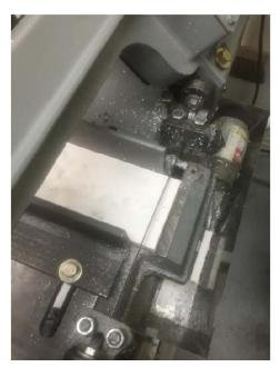
I started by sawing ½" wide strips of the expanded PVC on my horizontal bandsaw. Laying the stock flat helps give a square cut.
