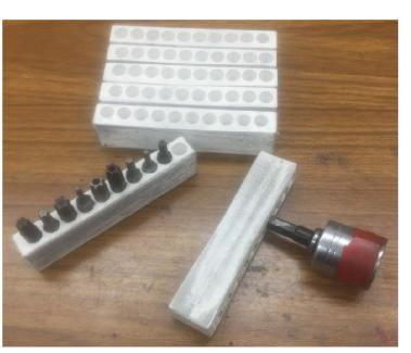
Next find the hex bit or adapter with the tightest fit. Press it into each hole to form the hex recess. You may need to move it in and out plus twist it slightly before it stops grabbing.
