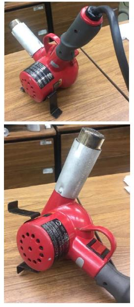
I own a very capable hot air gun<sup>2</sup> which is useful for resizing heat shrink tubing and reworking heat glue. It is a nice step down from my MAPP torch.
