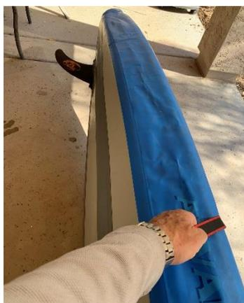
When I am at the water's edge, I slip on this strap, which is a loose fit. I can then place the kayak on the starboard gunnel with the hull next to me, steady the kayak with my right hand by holding onto the strap, and install the skeg with my left hand.
