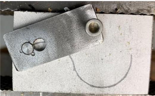
Then I dropped the guide into the hole and used the handle to rotate it until the line was centered in the hole. Then I drilled the next hole.
