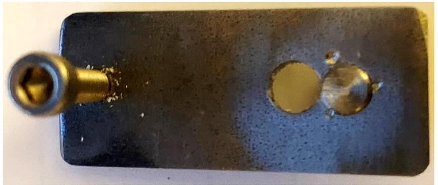
I drilled two 3/16-inch holes separated by 0.213-inches. This is the diameter of a #3 drill which I used as a spacer. Then I drilled and tapped a 6-32 hole to accept my little handle.
