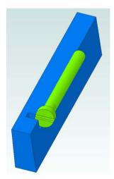
You are looking down on the Y axis gib. I have extended it from the apron so you can clearly see how the retaining screw works. Well, sort of works. Actually, barely works. The problem is that the gib can slide in and out as the apron moves. This causes the Y ways to over tighten as the apron moves away from the column and to become loose as it moves towards the column.
