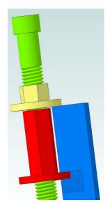
"Replace the inner nut with a fabricated part that threads onto the bolt. This part incorporates the inner flange that engages the outer edge of the notch in the gib, and has a hex that extents outward along the gib. The hex allows turning the inner flange using an end wrench, without the teasing with screwdrivers etc. in the table recess."
