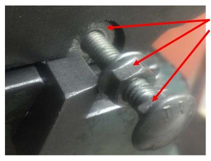
My solution consists of two flange nuts and a bolt. The bolt is first fitted with the nuts as shown. Then I screw down the bolt until it bottoms out eliminates backlash between the bolt and its threaded hole. Then the gib is positioned as the flange nut within the recess is spun out. Since this nut is not touching the gib, it is easy to turn with the end of a screwdriver. I turn until it contacts the face of the slot
