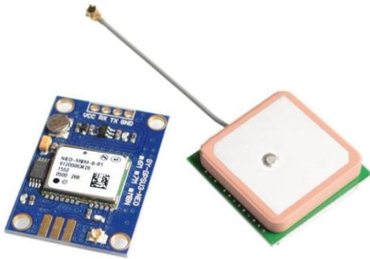
Devices are available for surprisingly little money. A simple Global Positioning System (GPS)<sup>2</sup> receiver, including antenna, can be bought for around \$4, including shipping from China. They use the USA's constellation of navigation satellites and is typically accurate to  $\pm 10$  meters.
