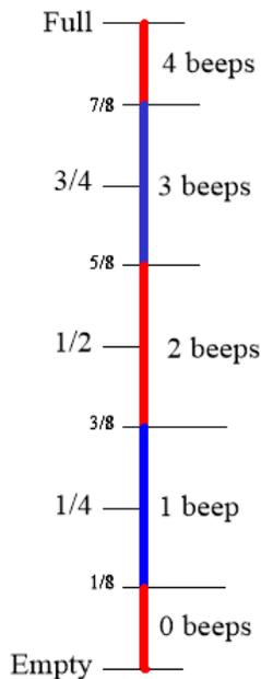
The number I need to convey to the user is the fraction of the remaining energy in my eBike's battery. Remember, requirement number 2 is to have minimal training of the user. In other words, the series of beeps should be painfully obvious.
