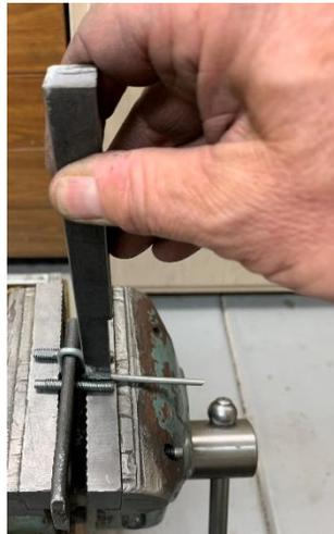
After tightening the vise, I'm ready for my next bend. I use the hammer to start the bend but then move on to tapping my steel bar to insure 90°.
