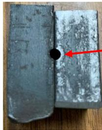
This was done on my drill press by clamping the stock plus some scrap of the same material face to face<sup>3</sup>. Then I drilled a 9/64 inch through hole at the interface. It is essential that the top surfaces are flush or it can snap off the end of the drill. I used a spotting drill to ensure that the 9/64 inch drill would not walk.
