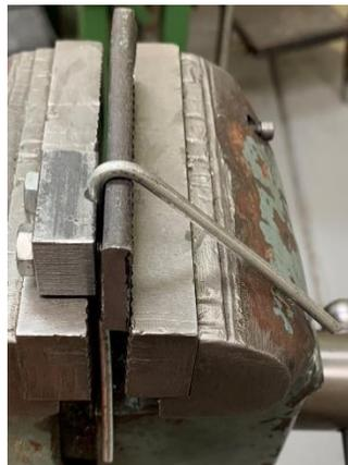
The wire is bent over as much as possible using my dead blow hammer.
