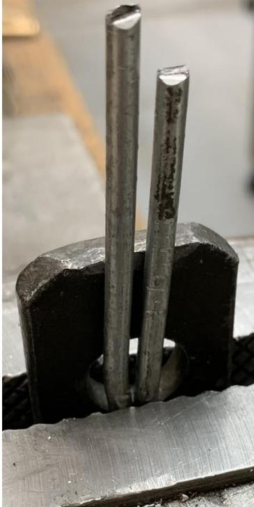
The formed wire goes back into the vise with the mandrel in preparation for making the hook.
