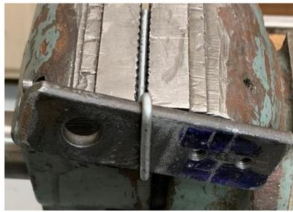
A gentle twist brings the wire ends into alignment.
