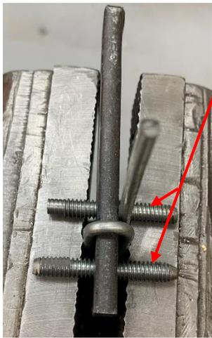
I then remove the clamping block and its bolts. Two lengths of threaded rod screw into the bolt holes.
