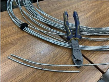
I bought a large coil of 0.144 inches in diameter galvanized steel wire from Home Depot a few years ago.
