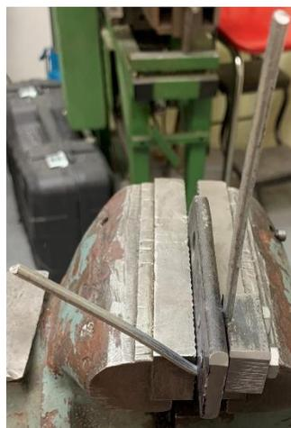
The mandrel is flipped over in preparation for bending the other end of the wire.
