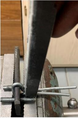
I again use the hammer to start the bend and the steel bar to finish it.
