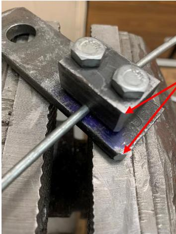
The clamping block with wire is secured to the mandrel with the two bolts.
