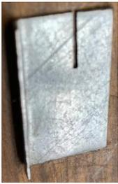
This is a piece of sheet metal that has a 1/4-inch bend along one side to make it easier to handle.
