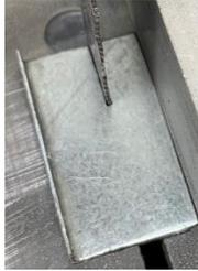
I made a cut with my saw the full depth of the blade about 3/8-inch from the edge. After deburring, I aligned a 1/4-inch wide parallel on the cut. Then I scribed a line with a knife for the full length of the metal. The distance from cut to edge is not critical, but being parallel is essential. As carefully as possible, I used tin snips to cut along that line. Deburr. OK, the tool is nothing to get excited about.
