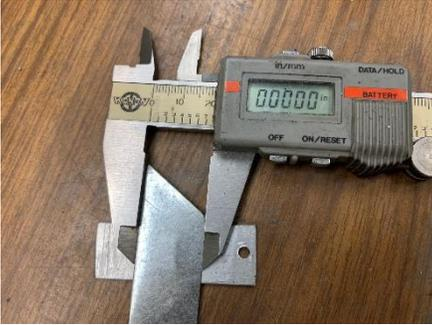
I zeroed my caliper at one end. The strip of metal enabled me to keep the jaws flat.
