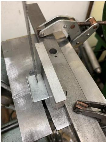
The value of this tool becomes evident when I align the fence. It is easier to see the edge of the tool than to sight the flank of the blade. I can hold down the tool, drop in a spacer, and then slide the fence in snug. Clamp the fence in place, remove the bits, and I'm ready to go. *The trick is to not press on the edge of the tool, which can cause the blade to twist or deflect.*
