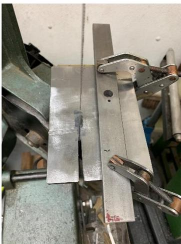
It is pleasing to my eye to see my fence parallel to the side of my bandsaw table. But as I got into the task of twisting the blade an additional 4°, I quickly realized it was not worth the trouble.
