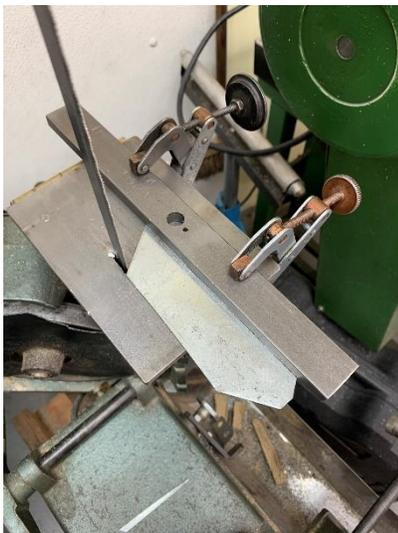
What happens if the flank of the blade is not parallel to the fence? The material being cut may be pushed into the fence and bind up or pull away from the fence. Either way, the result will be a cut that curves away from the intended path.
