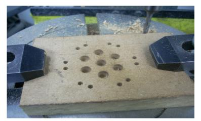
The RT will be moved to 0 first. I then move +/- 8.2 degrees from this point. Advance to 60 degrees and again drill +/-8.2 degrees from this point. In no time I have drilled the 6 sets of holes.
