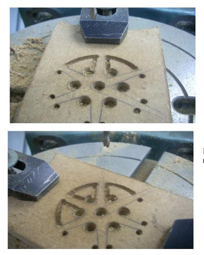
I cut my first spoke plus cut part of the perimeter. Notice the overshoot on the far end of the left flank of the spoke. I got one of the angles wrong. As with any project with so many steps, it only takes on mistake to screw up the part. I'll try another spoke.
