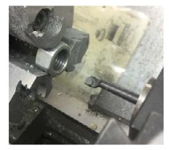
I put the nut in my lathe and bored in to half the thickness of the nut.
