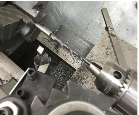
I drilled in about  $\frac{1}{2}$ ". At this point, I had a wall thickness of  $\frac{0.250-0.185}{2} = 0.033$ ".
