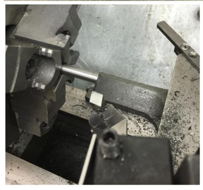
I chucked the steel into my lathe and faced off the end.
