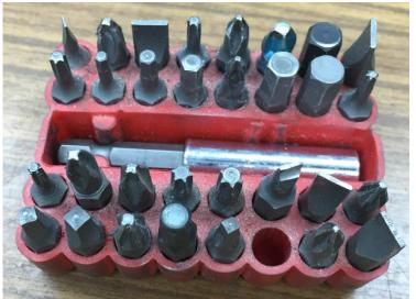
The first discovery was that I had a hex drive bit that was the same size as a 2-56 nut. When I measured the flat to flat distance, it turned out to be 0.185". That is also the same as a #13 drill. All I then needed was some scrap \(^{1}/\_4\)" diameter mild steel.
