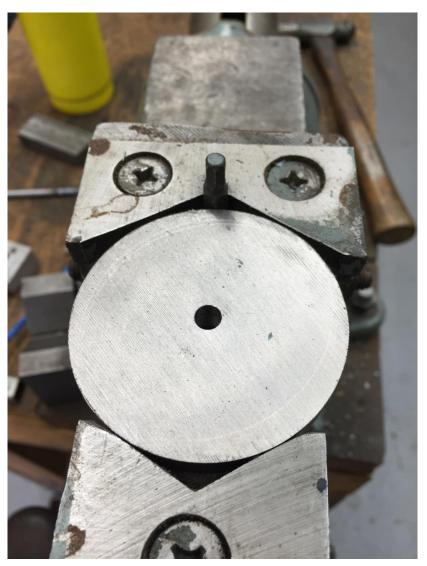
My bench vise has an odd set of jaws on the "bottom" side which lets me grab round things. This let me put the hex drive in the fixed jaw V and secure it with a round piece of scrap steel. In this way the hex drive is securely held vertical plus can't slide down because the vise jaws are supporting the end.
