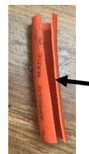
Notice that this piece of sheath is smooth on the inside. Better quality extension cords have internal ribbing which won’t fit well on the outside diameter of the damaged cord.
