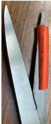
Since I have “The Disease”, almost nothing gets thrown away. That includes short lengths of extension cord. I took a 2-inch long piece, pulled out the wires, and cut it axially to make a patch.
