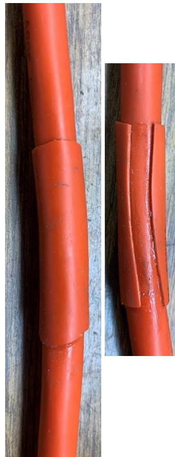
I centered the patch over the nick and wrapped it around the cord. A layer of thin steel wire wrapped around the path applied the necessary pressure. Wait the full curing time.
