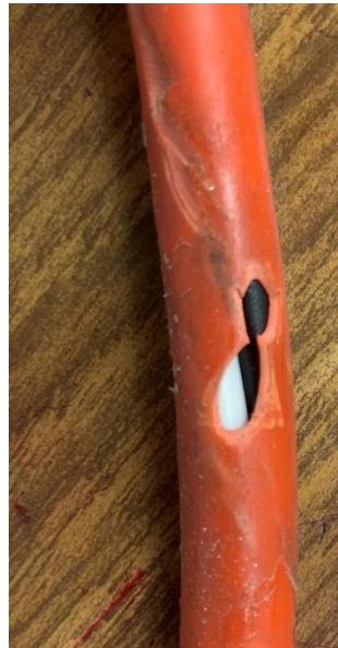
If just the outer sheath of a round cross-section extension cord has been nicked, people often wrap it in electrical tape. It looks good for a while but before long, the tape starts to lift. Bending of the cord loosens the wrap and dirt gets in. Before long, the entire mess falls off. Then you are back to having that exposed nick plus all of this sticky goo mixed with dirt around it. New tape won't stick to that. Gotta be a better way.
