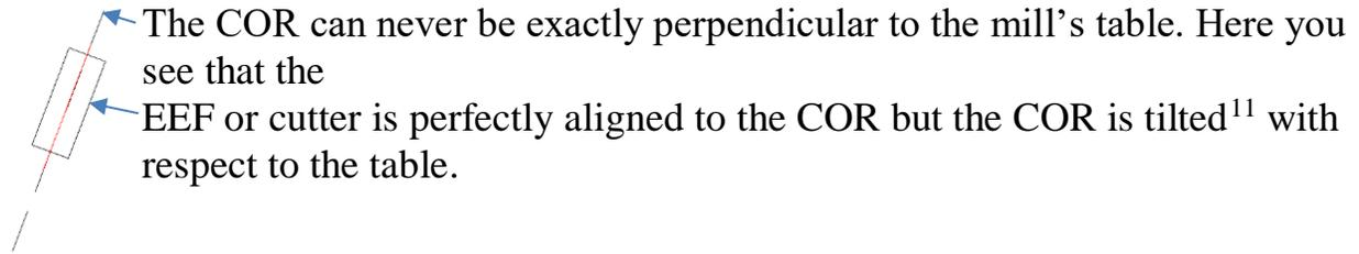
The COR can never be exactly perpendicular to the mill's table. Here you see that the EEF or cutter is perfectly aligned to the COR but the COR is tilted<sup>11</sup> with respect to the table.
