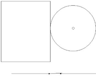
The instant the probe contacts the reference surface, we transition from an open circuit to a closed circuit.
