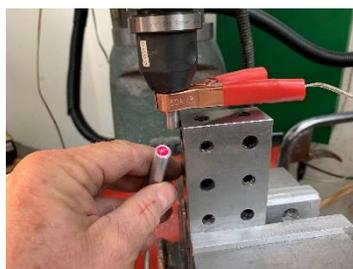
Proceed with finding zero on the X and Y axes. Always turn the spindle so the *A* reference mark faces the reference surface. If the probe is removed from the spindle, reinstall with the colored dots lining up.
