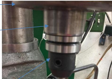
Attached to the bottom of the spindle is a means<sup>10</sup> by which cylinders like EEFs and cutters can be attached. Ideally, they attach in perfect alignment with the COR.
