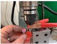
5. Turn the spindle so *A* faces the reference surface.
