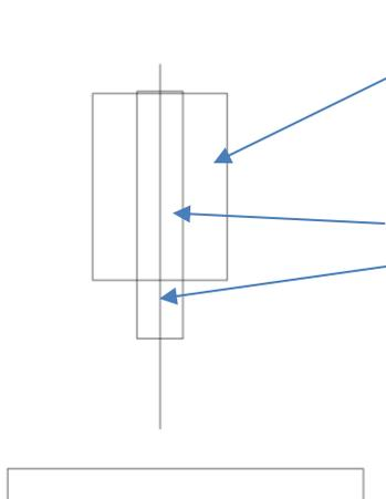
The mill has a Quill which ideally moves up and down. It carries the Spindle which ideally rotates around the COR. This enables the spindle to rotate plus move up and down.
