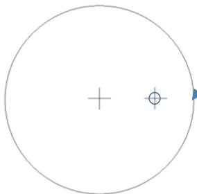
If I use this point to touch down on my reference surface, I'm closer than the radius of the probe.
