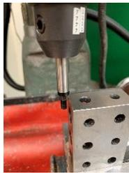
Using my Starrett mechanical edge finder<sup>6</sup> and again correcting for its probe radius, I read 5.4525 inches. Unpublished position repeatability of my machine has been measured at  $\pm 0.0005$  inches. Absolute accuracy with screw mapping enabled is  $\pm 0.001$  inches<sup>7</sup>. This means that error due to machine variation dominates and EEF error, with run-out compensation employed, is not significant.
