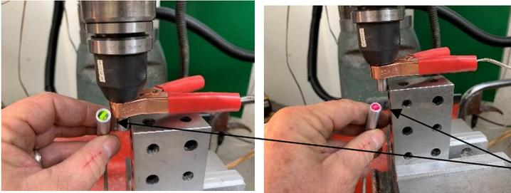
I was setting zero on my X-axis. The spindle was rotated so the A reference mark faced the reference surface, my 123 block. Then I had the CNC program automatically feed in until touchdown. Note that the LED changed from green to red.
