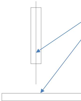
An ideal mill has its Center Of Rotation perpendicular to its table. The table's surface is parallel to the XY plane while the COR is parallel to the Z axis. In this way, a cutter rotating in alignment with the COR can be moved in XYZ space to cut precise shapes.
