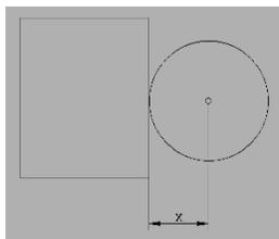
The important point here is that run-out causes the EEF probe<sup>12</sup> to act like it has a radius different than actual. When detecting touchdown, this misalignment can directly contribute to error in the COR to reference surface distance. That causes our zero point on this axis to shift.
