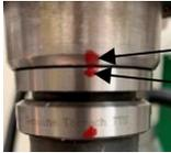
4. Place a single colored dot on the spindle that lines up with *A*. I have added a second dot on the top of the collet to ease alignment.
