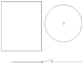
Given that the reference surface and EEF probe are clean, there is no more accurate method for sensing touchdown. We essentially have an electrical switch which is either open or closed<sup>9</sup>. The reference surface is one contact of our switch and the probe is the other. When the EEF is not touching the reference surface, the switch is open.
