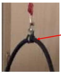
An insulated clamp goes around the charging cable and is supported by the rope. The clamp is just tight enough not to slide.
