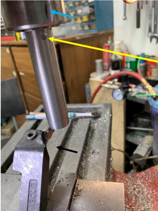
This time, I decided to put my lathe cutter in my mill vise (black arrow) and machine the reference surface in place. I drilled a shallow hole in the side of some  $\frac{3}{4}$  inch drill rod about 2 inches from one end and filled it with red paint. This dot lines up with an engraved line (blue arrow) that is aligned with a pin inside the spindle.
