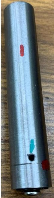
My probe<sup>2</sup> uses some of this  $\frac{3}{4}$  inch drill rod. I faced the end on my lathe and sawed off about  $\frac{1}{2}$  inch of it. Then I faced both the new end and the rough-cut face of the puck. These faces had a mirror finish thanks to my [Diamond Tool Holder](#).
