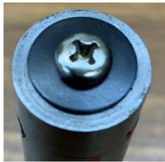
I secured the puck to the shank with a [Belleville washer](#) and a screw. This gave me plenty of friction between the puck and the shank without locking them up.
