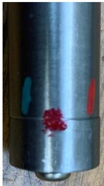
I first put red lines, 180 degrees apart on the end of the shank. Green lines were offset 90 degrees from them. With a red line at the DTI, I zeroed the indicator. Then I turned the spindle to the other red line and read the change. Finally, I divided this number by 2.
