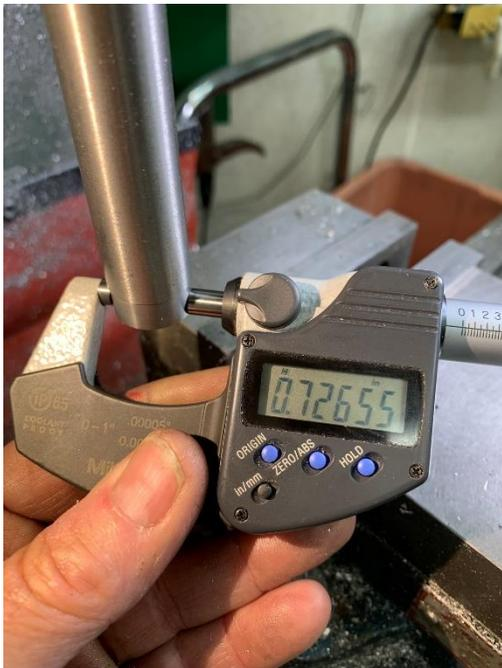
I measured the resulting diameter and found 0.72655 inches. This means that, on average, I removed about 0.012 inches from the radius.
