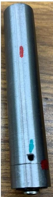
There is one more red line. The spindle has a pin inside of it that engages with the adapter. I have a red line on the outside of the spindle at this location. I align this red line with the red line on the shank. This minimizes any TIR in the shank and adapter.
