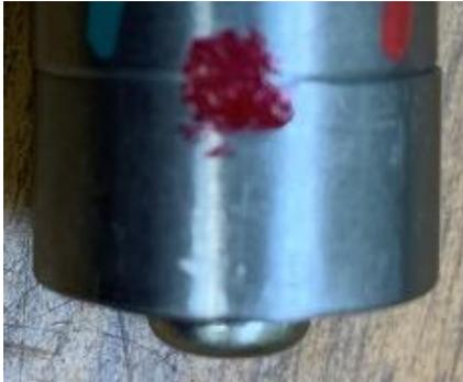
With alignment complete, I added dots of red paint across the shank/puck gaps. They will tell me if excessive side force was applied that shifted the puck. So far, so good.
