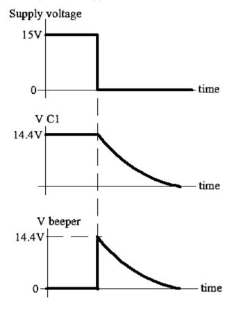
When the supply voltage has been at 15V DC for a long time, C1 charges up to about one diode drop below 15V. Call it 14.4V. Diode D2 conducts current through R1. The beeper sees about zero volts.
