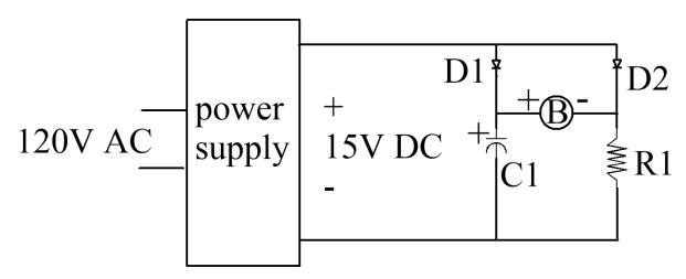
On the left is a wall wart that converts 120V AC into about 15V DC. D1 and D2 are 1 amp diodes. This is far more than I need, but I had them on hand. C1 is 1000 uf 30V and R1 is 220 ohm  $\pm 10\%$  2 watts. The symbol with the B in the middle is a piezoelectric beeper. This one has a built-in circuit that causes it to warble when power is applied. It works over a wide voltage range of 5 to 30 volts.
