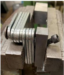
The next evolution of the design was to integrate the jack into the stack of spacers. This was done by adding a  $\frac{1}{2}$  inch by  $\frac{1}{2}$  inch bar to the stack. The bar contains the angled screw so I now have one assembly. The bar was also drilled and tapped  $\frac{1}{4}$ -20 to accept the long bolt. In this way, the spacers are secured without having to contend with the bolt head interfering with the angled bolt.
