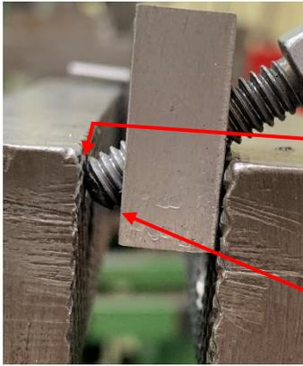
My variable thickness packing consists of a block with a screw through it. There are a few subtle design elements:
