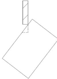
If done on my mill, I would have first used an end mill to cut a flat surface on the tilted block. Then running the drill would not have been done on a sloped surface.
