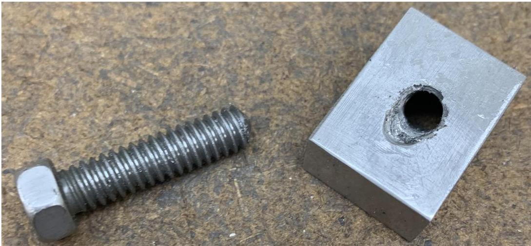
This is a proof of concept so I used an aluminum block and a 1/4-20 bolt. The bevel on the bolt was formed freehand on my belt sander.
