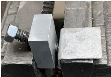
This was easily solved by dropping in a thin piece of aluminum bent into an "el". Now the bevel turns in a depression lined with soft aluminum.
