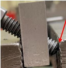
After gaining some experience with this tool, I realized that the bevel on the end of the screw was being chewed up by the sharp and hardened surface of the fixed jaw.
