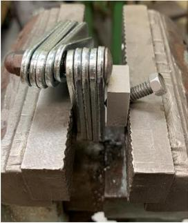
I found it easy to place my jack on the movable jaw and drag the stack of spacers into the remaining space. Those spacers that fit the void flopped in while the rest stacked up on top of the fixed jaw. So while this arrangement contains more parts, it is much easier to use.
