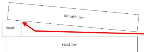
Without the packing, the movable jaw will tilt relative to the fixed jaw and the clamping action will be along one vertical line rather than across the face of the stock. The part can easily slip regardless of how much force is applied by the jaws.
