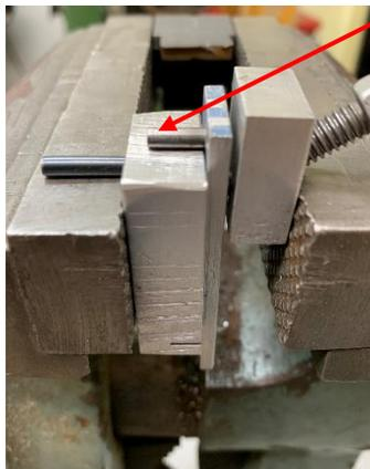
The roll pins are a quick and dirty way to reduce the chance of a block dropping down through the jaws before being tightened. If I change to steel blocks and put a magnet in each one, it should be easier to manage.
