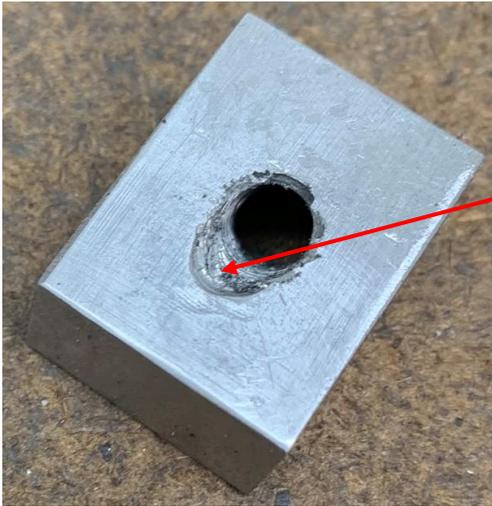
On my drill press, I first drilled down about 1/8 inch with my #4 with the block flat on the table. Then I tilted the block and drilled through with the same drill. This reduced side movement but did not eliminate it. You can see how the hole was a little buggered up. Not pretty but certainly functional.
