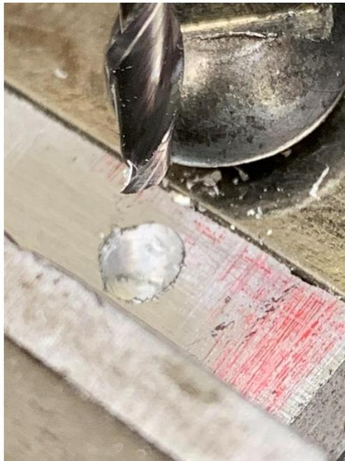
When the end mill cut a full circle, I was done. See the surface, directly under the center of rotation? It is parallel to the drill press table.
