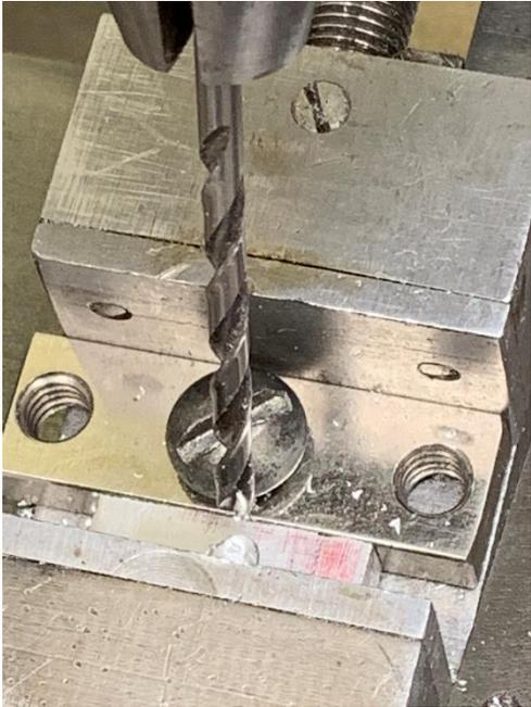
I replaced the end mill with my 1/8<sup>th</sup>-inch drill and finished the job.
