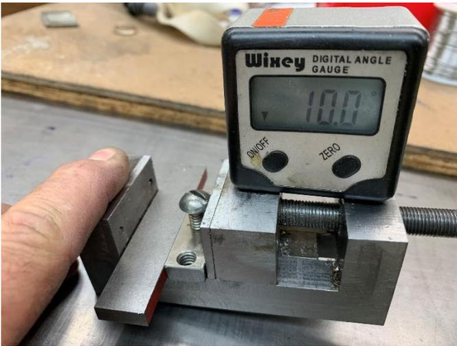
Then I turn the screw until the needed angle has been achieved. I can then transfer the vise with support leg to my larger vise and secure it.
