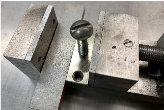
Start with a piece of scrap steel that has been drilled and tapped  $\frac{1}{4}$  - 20. Then thread in a screw. I place the assembly next to my stock and tighten the vise.
