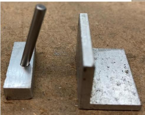
A 1/8<sup>th</sup>-inch dowel pin smoothly fits into the hole.
