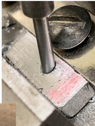
The spud went straight down the hole. This proves that the hole location did not shift during drilling.
