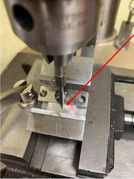
Before clamping the part in my tilted vise, I center punched the hole's location. After clamping, I used my spud to align the punch mark with my center of rotation. Since the punch mark is very shallow, little shift in location is introduced by tilting the stock.
