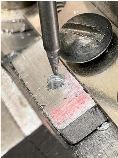
Installing my 1/8<sup>th</sup>-inch diameter spud, I lowered the quill and noted any deflection.
