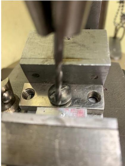
Next, I installed an end mill into the chuck that is at least as large in diameter as the hole I want to drill. Here you see a 1/8<sup>th</sup> -inch diameter end mill. It easily deflects as it cuts on the sloped surface but, if you go slow, it will return to true. No such problem with 1/4-inch end mills.
