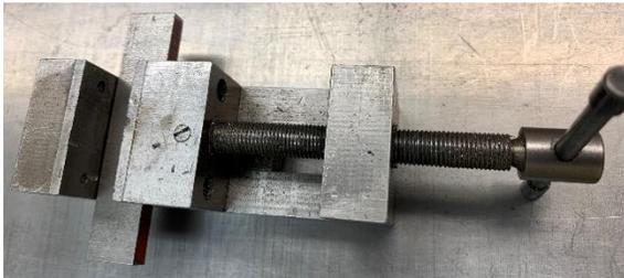
For small parts, I like to use my home made machinist vise. It gets clamped into my larger vise which, in turn, is clamped to the drill press table.
