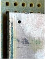
I start by selecting a hole location near a corner of the circuit board. It is carefully drilled free hand with my Dremel drill press.
