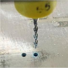
Next, I lift up my circuit board until the locator pins disengage from the perf board. I drop it down in the set of holes adjacent to the last set. This placed my drill 0.1 inch to the right of my first hole. Without needing to align the drill better than to the nearest 0.1 inch, I drill down and am confident that I am on grid.
