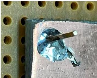
The pin is fed through the circuit board and into a piece of perf board below it. The perf board is flat on the table. This sets the stick-out of the pin at the same thickness as the perf-board. I then solder it in place while keeping the pin as vertical as possible. *You may have to resolder the pin if it is not vertical.*
