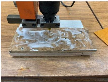
The perf-board was glued to the MDF using white Elmer's Glue. This has a few advantages. First of all, I can get the perf-board off of the table when it is worn out by pouring water on it. The glue is water soluble. Second, since no fasteners were used, I have access to every hole on the perf-board. And third, I have some work time before the glue sets.
