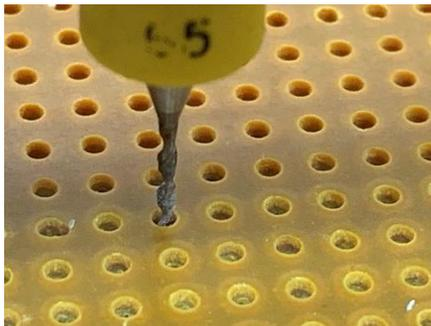
During the glue's work time, I slid around the perf board until I could lower the drill down through one of the holes. Alignment is critical here so I took my time. Note that the drill diameter matches the perf board which helps a lot.
