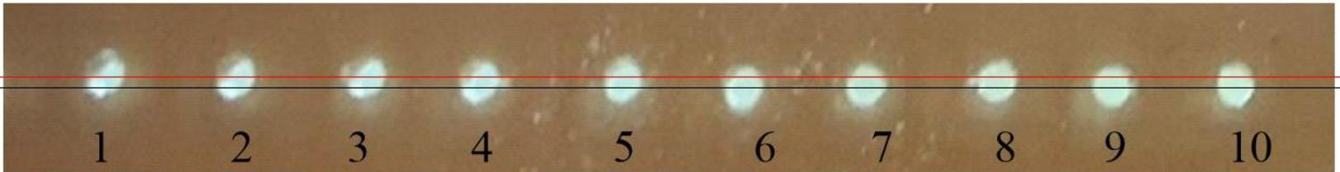
Holes 1 through 5 are centered along the red line. Holes 6 through 10 are centered along the black line. These holes are 0.04 inches in diameter and on 0.1 inch centers.
