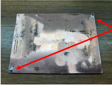
I took a piece of scrap copper clad board and installed pins on opposite corners. These pins are on the 0.1 inch grid of the circuit board but no artwork was etched.
