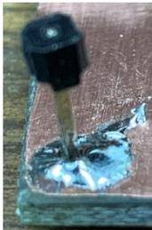
The plastic collar that is part of the connector makes a nice handle on the top of each pin.
