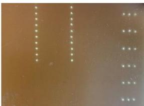
Ah, this is much better! See how all the holes are in a nice straight line and on grid. The alignment is good enough that sockets smoothly drop into place. The parallax problem has been eliminated and the entire process is about ten times faster.
