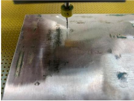
I drop the circuit board down on my perf board and move it around until my locator pins drop into holes near the position of my first hole. A little care must be taken to be sure the board is square to the perf board grid of holes.
