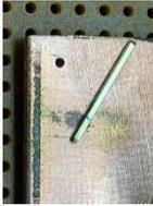
The tiny drill cuts a hole that it is a snug fit on a connector pin. These are the same pins that I use for all board mounted connectors and for component sockets.
