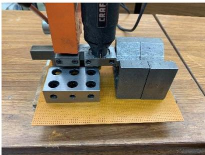
Then weights were placed on the perf board until the glue dried.
