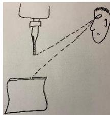
Parallax makes it nearly impossible to align the end of the tiny spinning drill with an equally tiny spot on the board. Consider that the drill is around 0.04 inches in diameter and is around ¼ inches above the surface. I must carefully lower the drill to reduce parallax yet not touch-down until I'm at the right spot. Time to look for a better way to do this.
