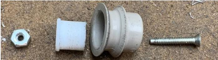
I'm using a nickel-plated flat head screw and a nickel-plated nylon lined lock nut. These will be replaced with stainless before they start to rust.
