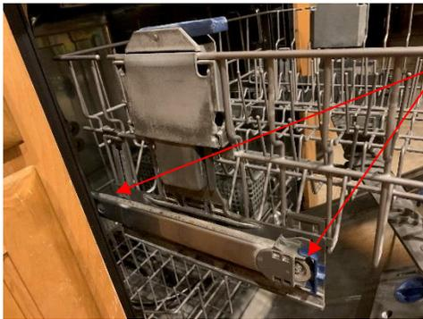
The weak links on my KitchenAide dishwasher are the wheels that carry the top rack. The wheel carrier is made of resin plastic which holds up well to the hot water but is brittle. This video explains the problem and how to replace the carrier:
