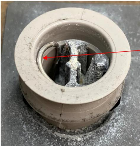
Tiny spring fingers hold the wheels on and when they break off, the wheel follows. Here you see one finger gone but I have replaced it with a piece of stainless steel wire. This works well as long as one finger remains. Eventually, both fingers break off.
