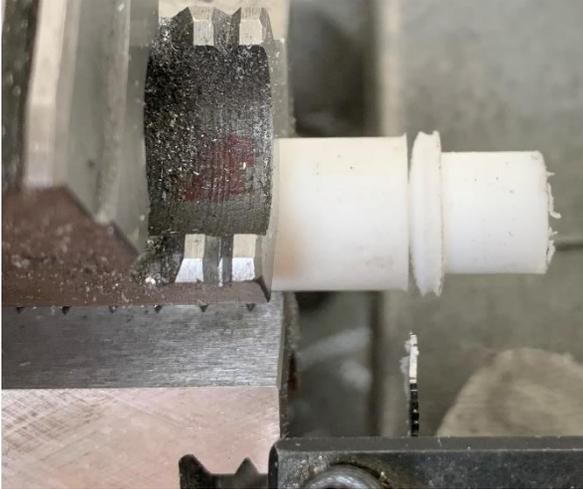
I took the dimensions from the spacer and turned the new axle. Here you see the overall length complete along with the outside diameter of the axle. I parted off with my hacksaw blade grooving tool<sup>2</sup>. The nylon squirms so I ended up with a crowned top.
