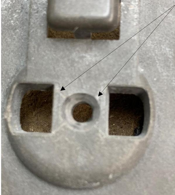
The first step was to scribe lines between the two cut-out areas in order to locate my new mounting hole. Then I used my 1/8" spotting drill at the intersection and followed with a #27 to give me a 6-32 clearance hole. Using a countersink mounted in a brace-and-bit, I carefully cut the recess. The screw must be flush with the surface to avoid binding. Fortunately, there is enough thickness to sink the screw head and still have strength.
