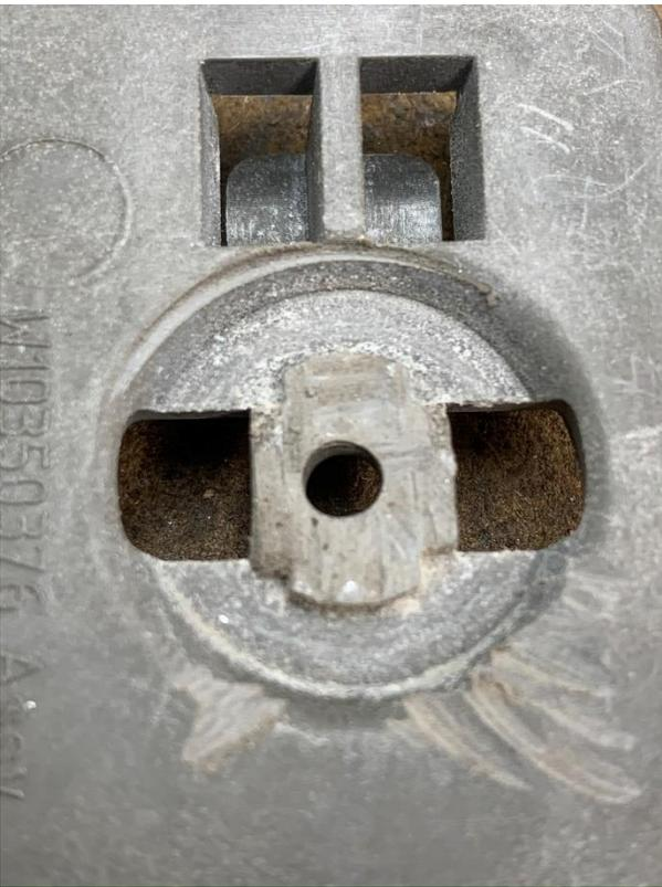
Next, I ground off the post in the carrier with a Dremel cut-off wheel. My goal was to establish a flat surface and not tear up the remaining plastic too much.
