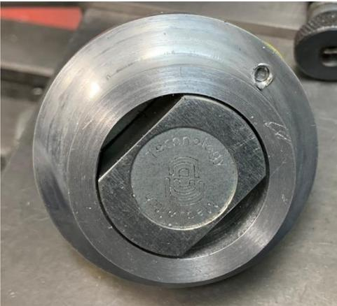
The length of the smaller OD permits about 10 thou of the Magswitch to be proud. This is necessary for maximum holding force.
