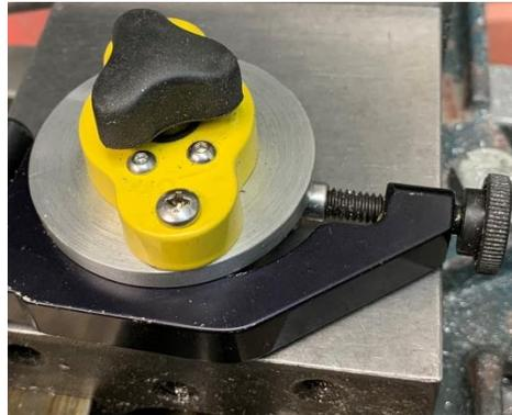
Be mindful that this length must be sufficient to permit the knobs to turn without binding on a mounting surface. Here you see the knob hanging over the edge of the surface. I had to thin the larger OD to raise it up about 0.1 inches.
