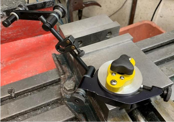
I turned a collar out of 6061-T6 aluminum. The smaller OD matches my spindle OD. The larger OD matches the Magswitches major axis width. The thickness of the larger OD is enough to accept three threads of my 6-32 mounting screws.
