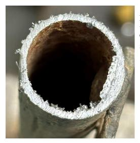
After sawing off the end of a piece of scrap ½" EMT, I am left with a variety of sharp edges that can easily cut through plastic insulation. It is standard practice, and code, to remove these burrs.
