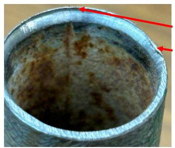
If I drill in too far, there is a risk of sharpening the face of the cut. Then, the file can fold over the sharp edge.
