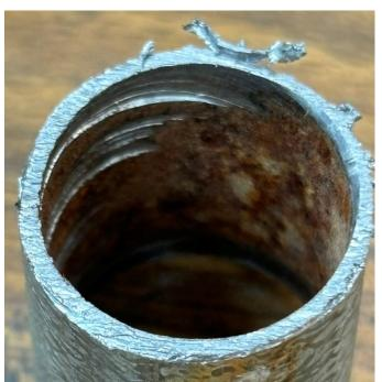
Here is the inside of a conduit after the inside had been "rotary deburred."
