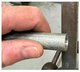
The outside burrs and face of the cut are efficiently deburred using a flat file.
